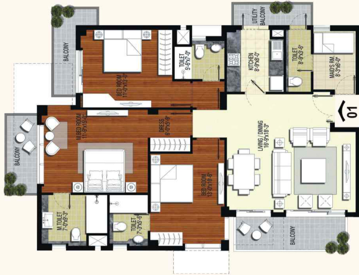
TOWER - A, B, C & D UNIT - 01 PLAN (EVEN FLOORS) SIZE - 1870 SQ. FT.
